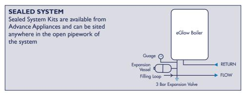
The eGlow boiler can only be configured into a sealed system. A sealed system kit can be purchased from Advance Appliances to make the job simple. An 8 litre expansion vessel is supplied with each kit but it should be noted that systems with high water content may require larger vessels. All heating systems must be isolated from the mains water supply after the system is filled.
